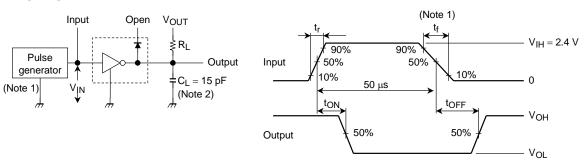
Note 1: Pulse Width 50  $\mu$ s, Duty Cycle 10%
