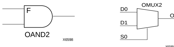
Figure 20: AND & MUX Symbols in XC4000X IOB
