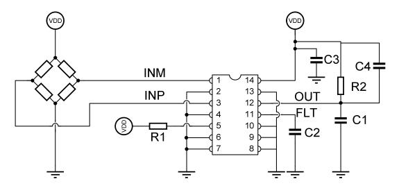
The external temperature sensor is only needed for applications where the temperature surrounding the customer sensor is different from the temperature surrounding the MLX90326. In the ratio-metric application mode, to keep the accuracy, the same supply should be used for the customer sensor, the MLX90326 and an ADC that makes the digital conversion of the analog output signal.
