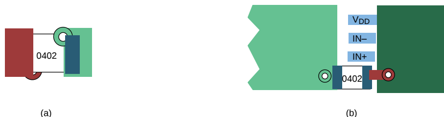
Figure 48. Typical Decoupling Capacitor Layouts
