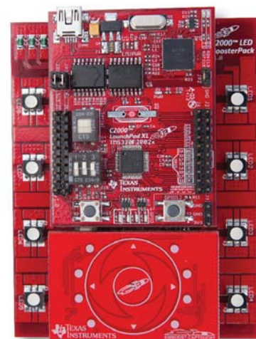
▲ Expand your C2000 Piccolo LaunchPad with application-focused C2000 BoosterPacks, which plug right into the headers. Pictured: C2000 Piccolo LaunchPad plus C2000 LED BoosterPack plus MSP430™ Capacitive Touch BoosterPack
