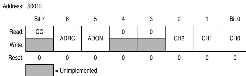
Figure 9-1. A/D Status and Control Register (ADSC)
