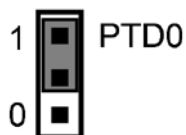
Figure 7-11: Accelerometer g-Select1 Jumper settings (J13)
