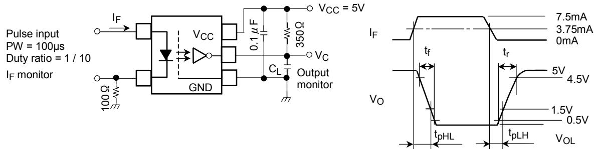
C<sub>L</sub> is approximately 15pF which includes probe and stray wiring capacitance.
