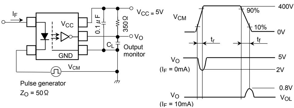
C<sub>L</sub> is approximately 15pF which includes probe and stray wiring capacitance.
