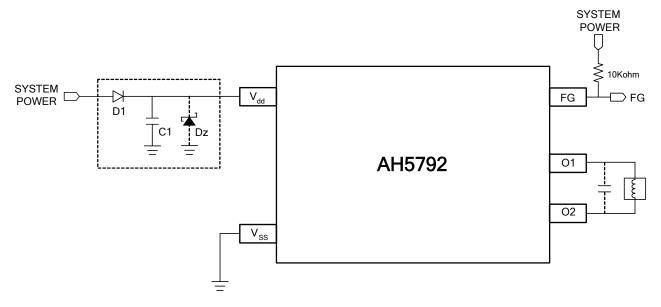
Notes: 1. Reverse connection of power supply may break the device. A countermeasure is needed such as using reverse power protection diode D1 between power supply and Vdd terminal. In such case of using reverse power protection diode D1 because of there is no way to return current to power supply, please take necessary measures like below.
