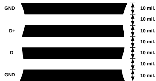
Figure 19. Arrangement of Signal Tracks
