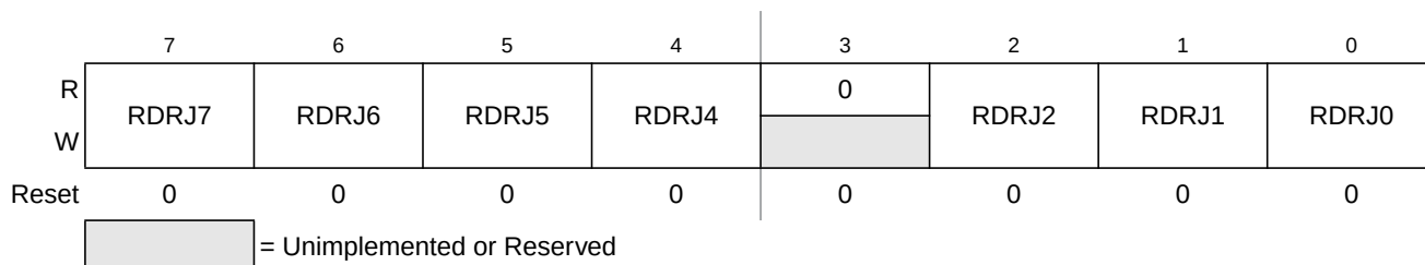
Figure 23-59. Port J Reduced Drive Register (RDRJ)
