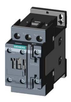
CONTACTOR, AC-3, 18.5KW/400V, 1NO+1NC, AC 220V 50/60HZ, 3-POLE, SZ SO SCREW TERMINAL
