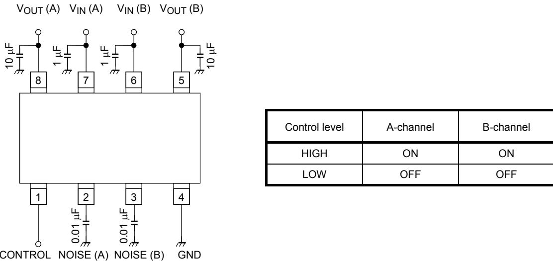
The noise capacitor should be connected to NOISE pin to GND for stable operation.
