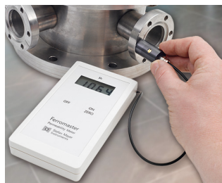
Ferromaster Permeability Meter
