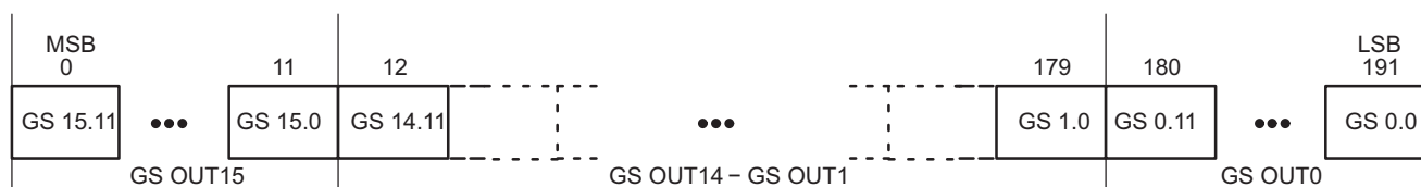
Figure 17. Grayscale Data Packet Format
