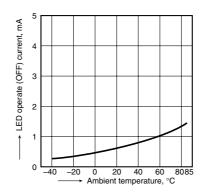
6. LED reverse (ON) current vs. ambient temperature characteristics Load voltage: 400 V (DC);
