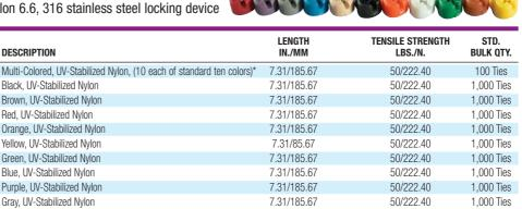
For use in temperatures ranging from -40° F to 185° F (-40° C to 85° C).
