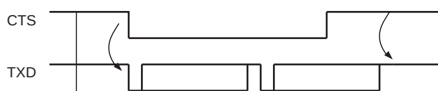
Figure 47-28: Transmitter Behavior when Operating with Hardware Handshaking
