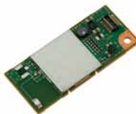
WLAN Original Antenna & Board to Board Connector
