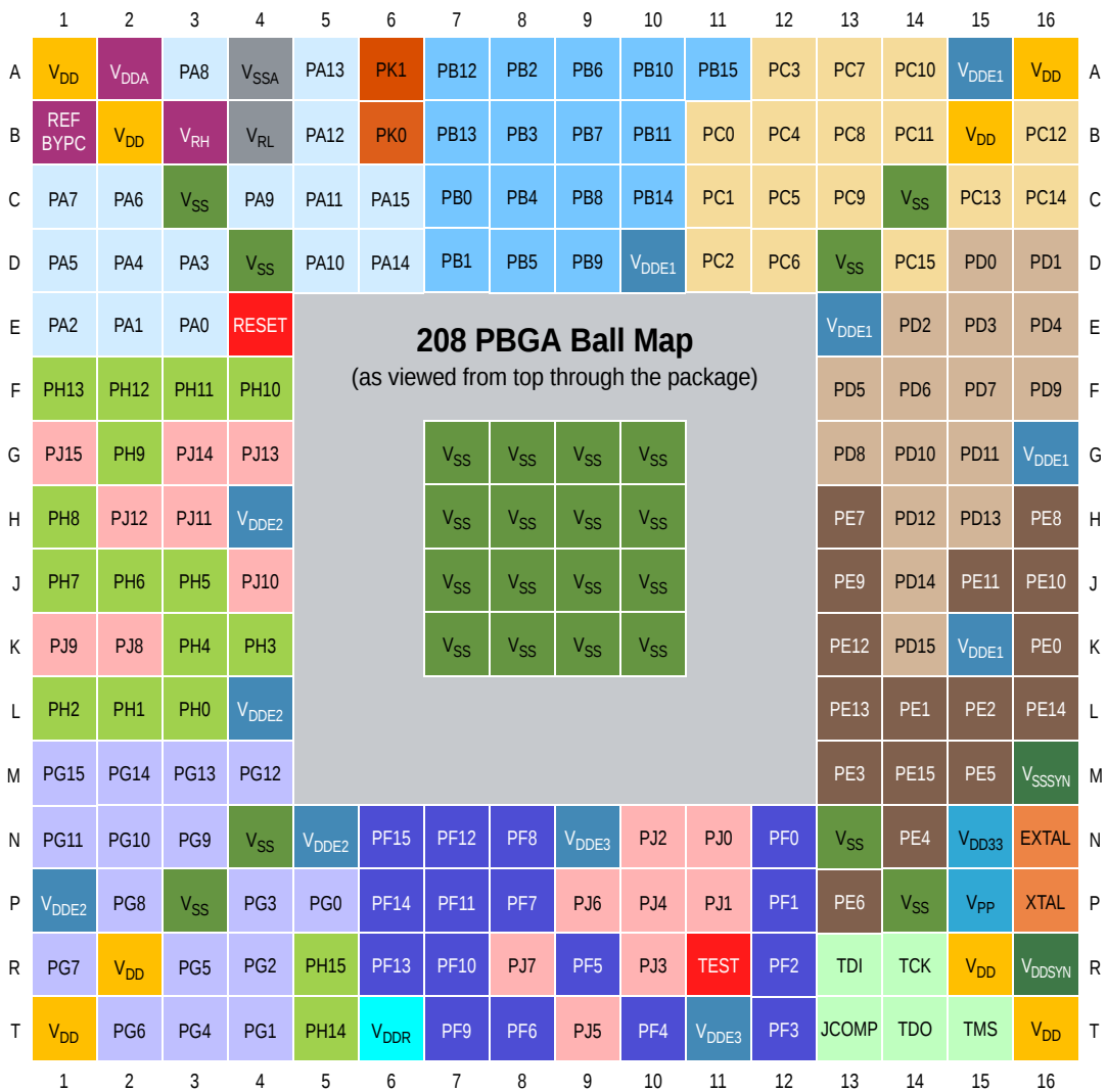
Figure 4. MPC5510 Pinout – 208 PBGA
