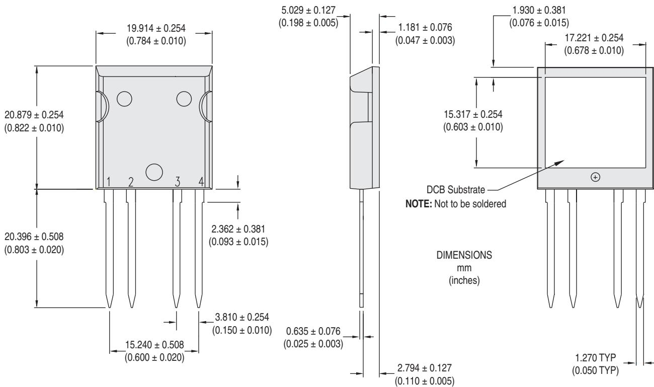
**NOTE:** Metallized external surface of DCB substrate maintains 2500V<sub>rms</sub> isolation to device internal structure and all external pins.
