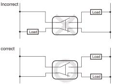
Connect the load to the same polarity.
