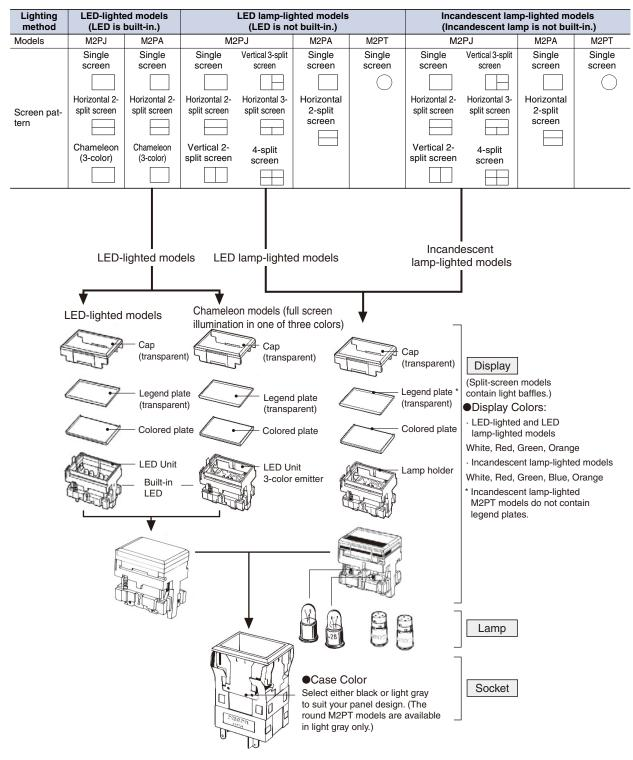
Note: The above diagram for LED lamp-lighted and incandescent lamp-lighted models shows the M2PJ model.
