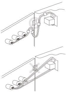
With miniature Switches, the gap between the terminals is very narrow. Use protective or heat-absorbing tubes to prevent burning of the wire sheath or shorting.
