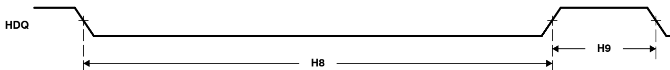
Figure 5–39. HDQ/1-Wire Break (Reset) Timing
