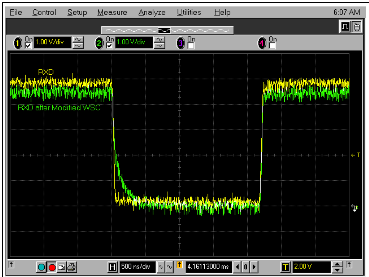
FIGURE 2-19: MCP2140A MODIFICATIONS OF MCP2140 WAVE SHAPING CIRCUIT
