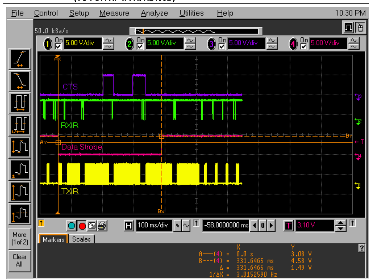
FIGURE 2-15: HOST CONTROLLER TRANSMISSION (S → P) OF A 250 BYTE PACKET (TO PDA HP IPAQ H2495B)
