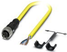
Sensor/actuator cable, 5-position, PVC, yellow, free cable end, on Socket straight M12 SPEEDCON, A-coded, cable length: 10 m
