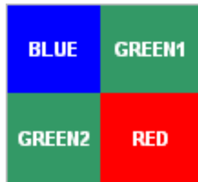
Figure 4. Color Filter Arrangement on the Pixels
