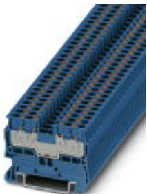
Feed-through terminal block, with widened marking grooves for TMT... Materials, Connection method: Push-in connection, Cross section: 0.14 mm<sup>2</sup> - 2.5 mm<sup>2</sup>, AWG: 26 - 12, Width: 5.2 mm, Height: 35.3 mm, Color: blue, Mounting type: NS 35/7,5, NS 35/15
