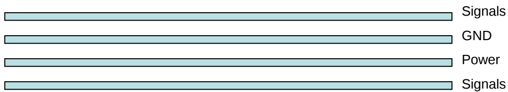
Figure 5: Typical 4-layer PCB construction
