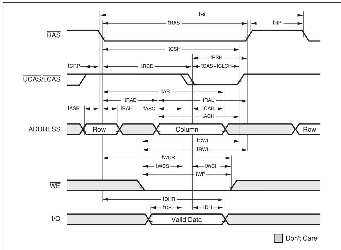
FAST-PAGE-MODE READ WRITE CYCLE (LATE WRITE and READ-MODIFY-WRITE Cycles)
