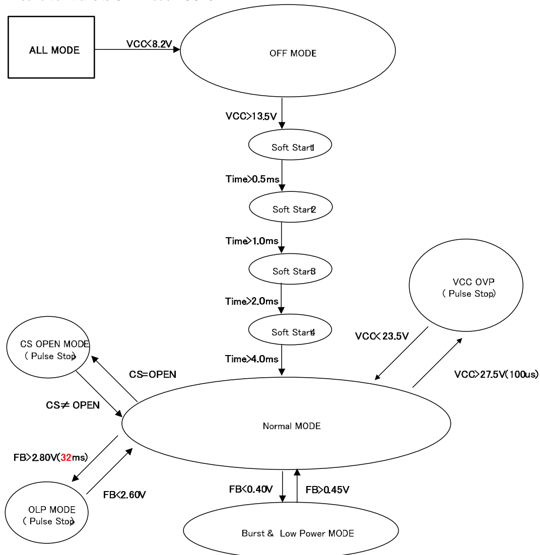
Figure 18. The sequence diagram (BM1PXX1 Series)
