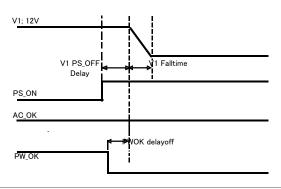
1. Note this characteristic is applicable for the main 12Vdc output shutdown from PS\_ON pulled high.
