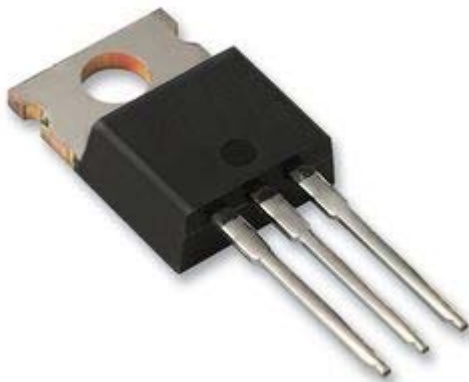
Fig. 1 Simplified Outline (TO-220C) and Symbol
