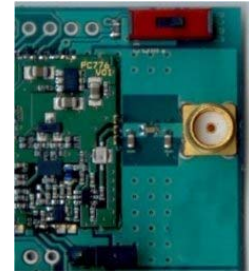
Figure 5. SMA connector for external antenna
