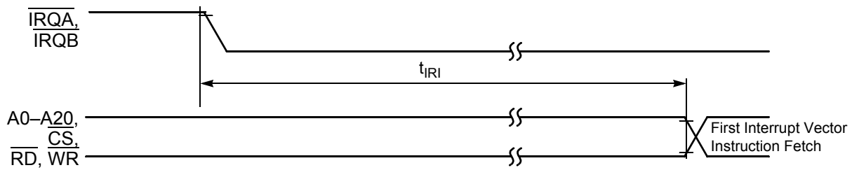
Figure 4-14 Interrupt from Wait State Timing
