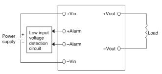
The input voltage detection output terminal (±Alarm) is a transistor output of a photo-coupler and it is insulated at the both input and output sides.
