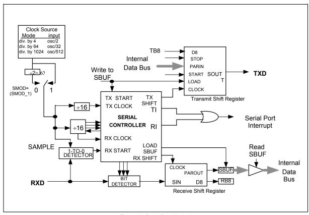
Figure 22. Serial Port Mode 2
