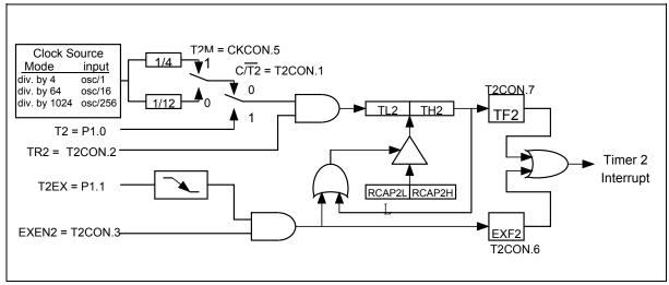
Figure 15. 16-Bit Auto-reload Mode, Counting Up
