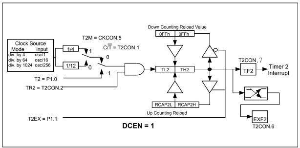
Figure 16. 16-Bit Auto-reload Up/Down Counter
