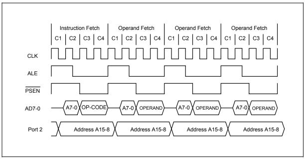
Figure 6: Four Cycle Instruction Timing
