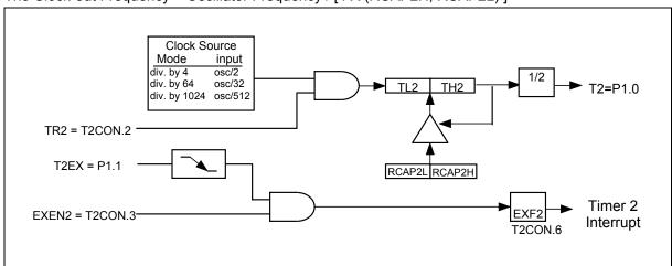
Figure 18. Programmable Clock-Out Mode
