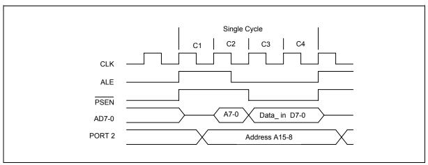
Figure 3: Single Cycle Instruction Timing
