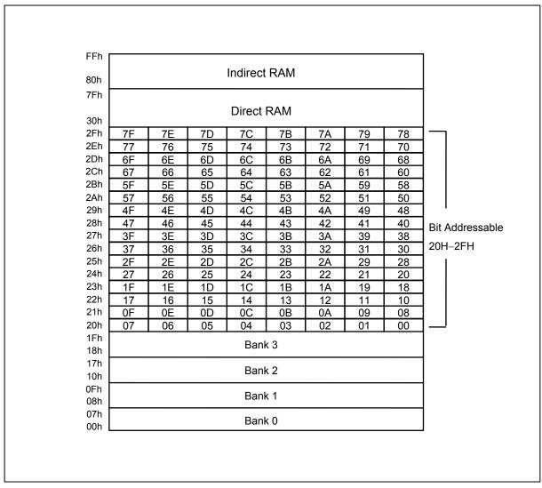
Figure 2. Scratchpad RAM / Register Addressing
