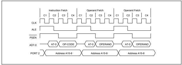
Figure 5: Three Cycle Instruction Timing
