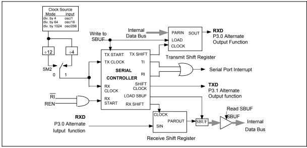
Figure 20. Serial Port Mode 0
