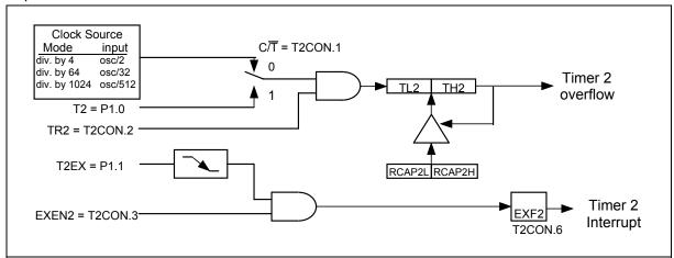
Figure 17. Baud Rate Generator Mode
