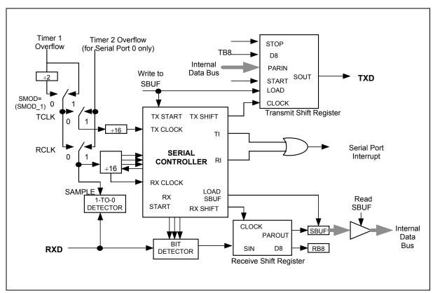
Figure 23: Serial Port Mode 3
