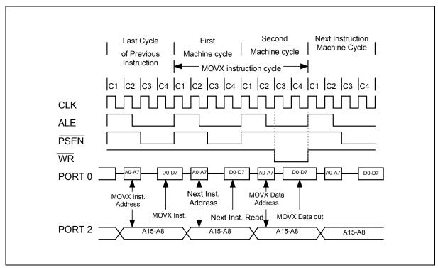
Figure 8: Data Memory Write with Stretch Value = 0
