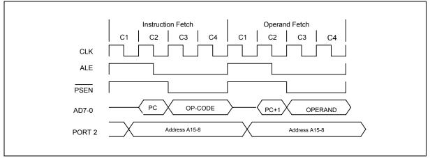
Figure 4: Two Cycle Instruction Timing
