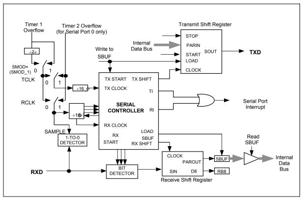
Figure 21: Serial Port Mode
