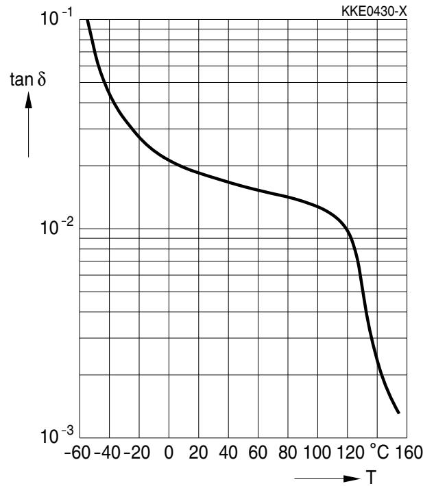
Dissipation factor  $\tan \delta$  versus temperature T for HighCV
