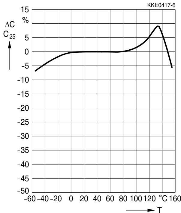
Capacitance change  $\Delta C/C_{25}$  versus temperature T for BME
