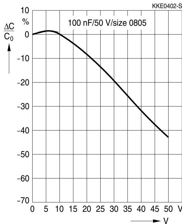
Capacitance change  $\Delta C/C_0$  versus superimposed DC voltage V for HighCV
