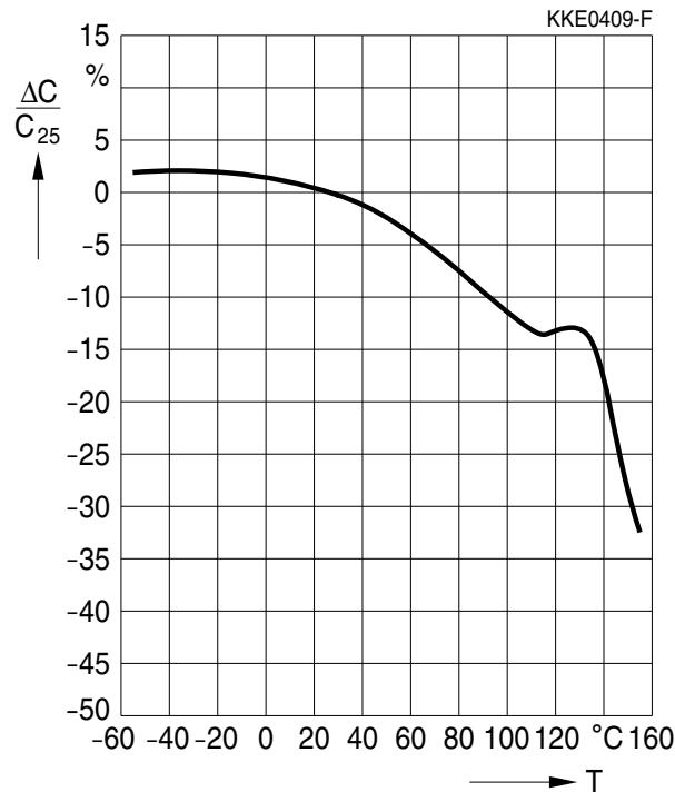
Capacitance change  $\Delta C/C_{25}$  versus temperature T for HighCV
