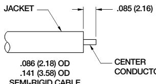
Strip the cable jacket and dielectric to dimension shown. Do not nick the center conductor.
