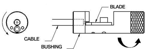
Insert the stripped cable into the bushing of the appropriate pointing tool until the center conductor just touches the blade. While maintaining light pressure on the center conductor against the blade, turn the tool in a counter-clockwise fashion as viewed from the bushing end of the tool. Continue cutting the center conductor point until the cable jacket bottoms out inside the bushing.
