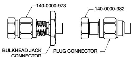
Attach the appropriate soldering mating fixture to the connector and tighten to a maximum of 8 inch pounds of torque.
