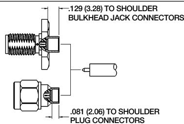
Clean all debris from the prepared cable and insert the cable into the connector, making sure that the cable jacket bottoms out against the internal shoulder of the connector body.
