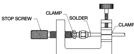
Insert the stop screw into the mating fixture. Clamp the cable and fixtured connector assembly securely in the soldering vise. Solder the connector body to the cable as shown, while insuring the cable dielectric expansion does not move the assembly. Allow the assembly to cool before removing the connector from the fixture
