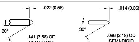
Bevel the entire diameter on the end of the cable center conductor until the point resembles the appropriate dimensional profile. This operation can be accomplished effectively by using the recommended center conductor pointing tool as described in step 4.
