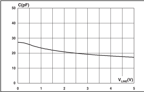
Figure 11. Junction capacitance versus reverse applied voltage (typical values, reverse)
