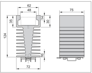
It is essential to use heat conduction foil or heat conductive paste between the solidstate relay and the heat sink.
