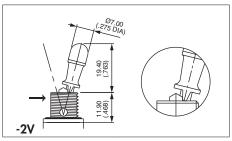
2 locked positions (function 6) Typical angle of throw: 26°
