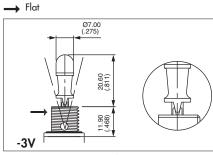
3 locked positions (functions 9 and 4) Typical angle of throw : 20°
