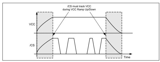
Figure 58b. Power-up, Power-Down Requirement
