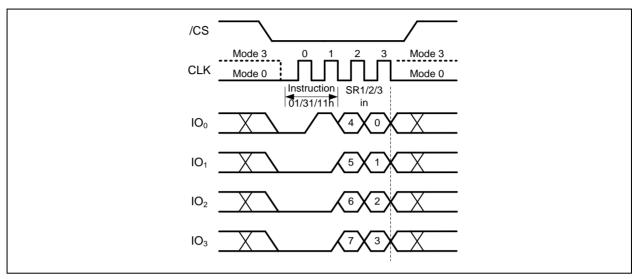
Figure 9b. Write Status Register-1/2/3 Instruction (QPI Mode)
