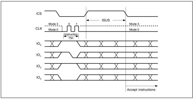
Figure 35b. Erase/Program Suspend Instruction (QPI Mode)
