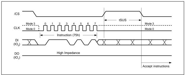
Figure 35a. Erase/Program Suspend Instruction (SPI Mode)
