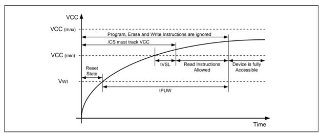
Figure 58a. Power-up Timing and Voltage Levels
