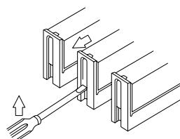
2. Both ends of the relay are to be secured firmly so that the socket hooks on the top surface of the relay.
