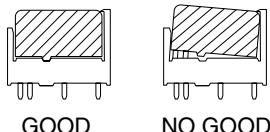
Notes: 1. Exercise care when removing relays. If greater than necessary force is applied at the socket hooks, deformation may alter the dimensions so that the hook will no longer catch, and other damage may also occur.
