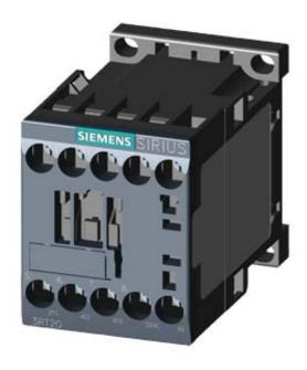
CONTACTOR, AC-3, 5.5KW/400V, 1NC, AC 220V 50HZ 240V 60 HZ, 3-POLE, SZ S00 SCREW TERMINAL
