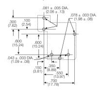
Only necessary terminals are present on single throw models and terminal code 4 models. Consequently, some holes will be unnecessary for those models.
