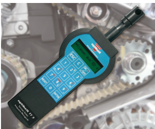
Pretension tester for V-belts and toothed belts
