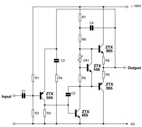
Depth/Echo sounders require high power linear amplifiers for driving the transducer. Since these amplifiers operate in pulsed mode, the average power dissipation experienced by the output transistors is low, but the value of the pulsed current can be very high. This would normally dictate that high power, large package power transistors would be required, which tends to increase the overall circuit size.
