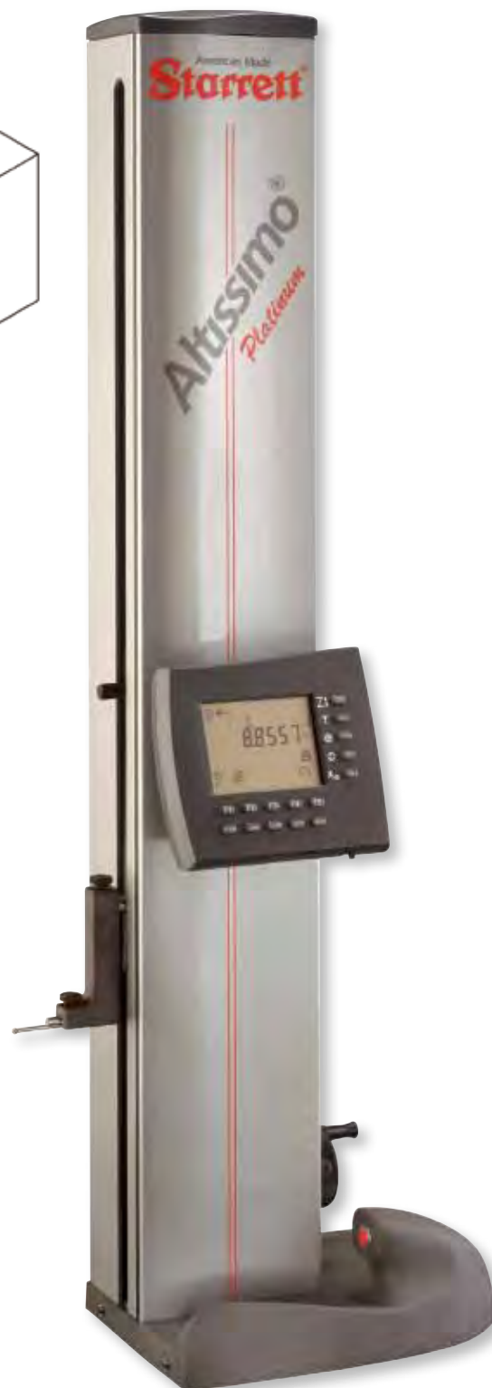
Interactive LCD with unique scanning meter for easy probe position viewing.
