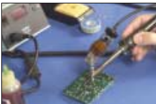
The WDD81V is shown here with the DS80 desoldering pencil.
