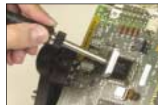
A SMT quad tip is used to desolder a quad flat pack.
