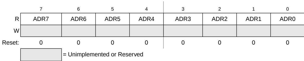
Figure 9-6. Data Result Low Register (ADCRL)
