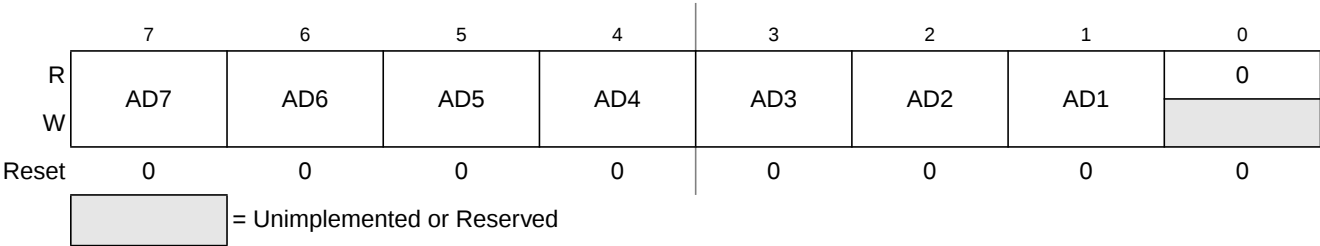
Figure 10-3. IIC Address Register (IICA)
